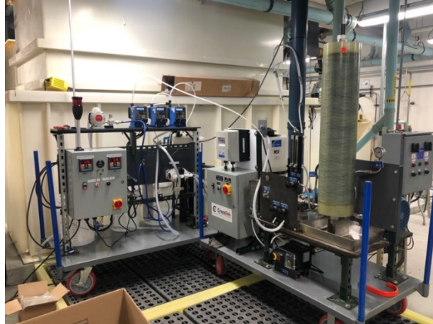
Figure 1: Crosstek Benchtop Disc-Tube Reverse Osmosis Pilot System
